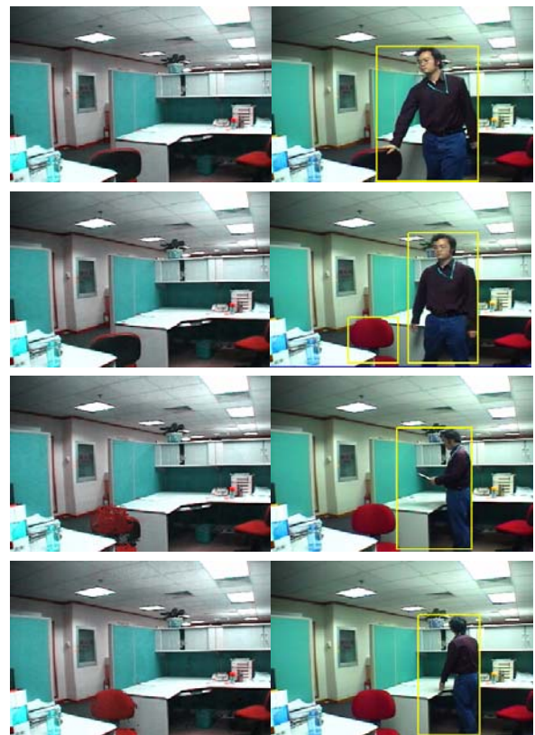
Figure 7. Left object, a person move a red chair into different place. These images are captured at frame #1, frame #13, frame #98, frame #189. The first column contains the background model. The second column contains the bounding box of the detected moving object.
