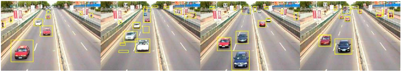
Figure 5. Vehicle segmentation for traffic video surveillance . These images are captured at frame #1, frame #78, frame#161, frame #236 separately. The first row contains the background model. The second row contains the subtraction image. The third row contains the moving object segmentation result. The fourth row shows the objects' position boxes calculated from the blob labeling results.
